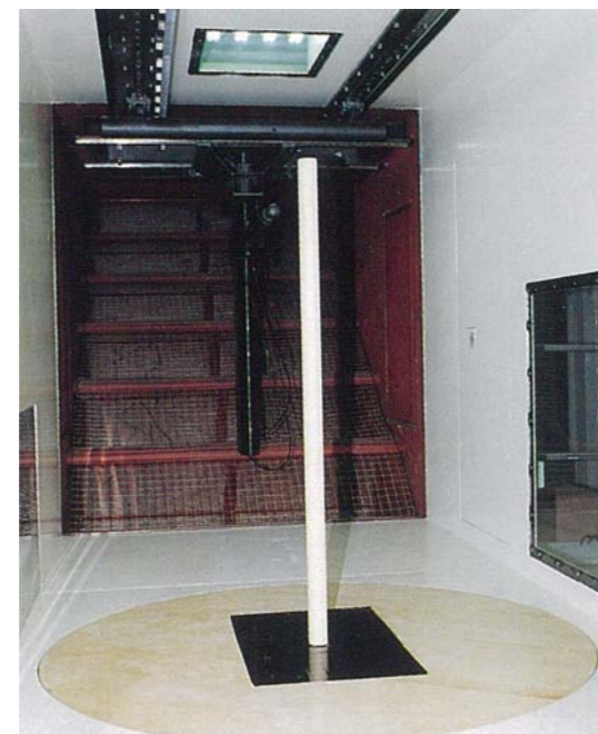
塔状円柱弾性模型実験 Elastic Model Test of Circular Cylinder Tower
