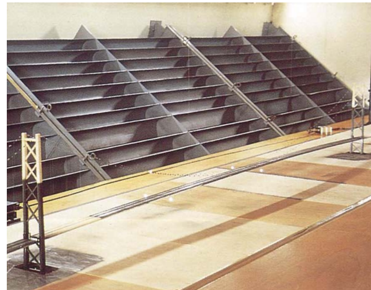
明石海峡大橋箱桁案全橋模型実験 Aeroelastic Full Model Test of Akashi Kaikyo Bridge - Box Girder Alternative
